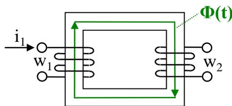
$$\begin{aligned} i_1 &= (1 \text{ A}) \sin(2\pi 50 \text{ Hz} \cdot t) \\ w_1 &= 10 \\ l_{\text{Fe}} &= 20 \text{ cm} \\ A &= 1 \text{ cm}^2 \\ \mu_r &= 5000 \\ w_2 &= 100 \end{aligned}$$
