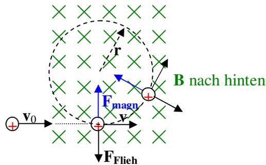
$$\mathbf{F}_{\text{magn}} = Q (\mathbf{v}_0 \times \mathbf{B}) \quad \text{und} \quad \mathbf{F}_{\text{Flieh}} = -m\omega^2 \mathbf{r} = -m \left( \frac{2\pi}{T} \right)^2 \mathbf{r} \quad \text{mit} \quad 2\pi r / T = v_0$$
