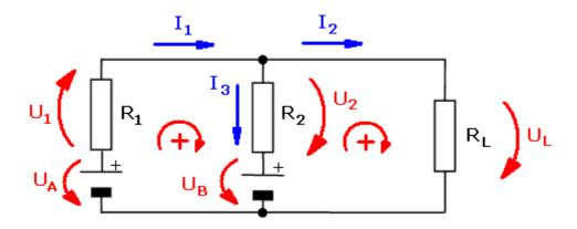
$$D = R_1 R_L + R_L R_2 + R_2 R_1 = 6*18+18*6+6*6 \Omega^2 = 252 \Omega^2$$
